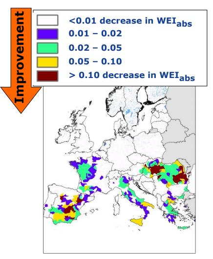
Showing changes if all irrigation is transformed to **drip irrigation**, increasing water efficiency from 83% to 93%
