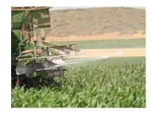
Tractor in field spreading differential N rate
