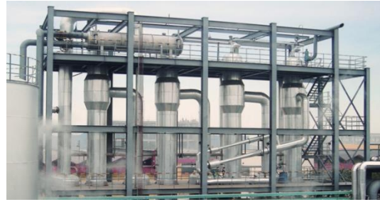
Figure F.25. TVR: Thermal vapor recompression process lxxi
