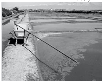
Figure F. 15. Crystalliser pond with floating fleur de sel in Noirmoutier, FR
