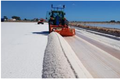
Figure F.18. Mechanical sea salt harvesting in SP
