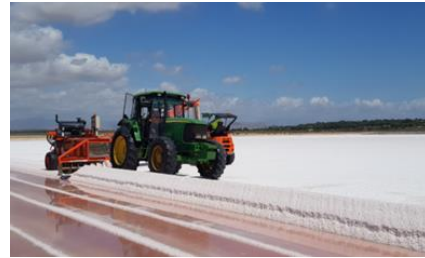
Figure F.19. Mechanical sea salt harvesting in SP
