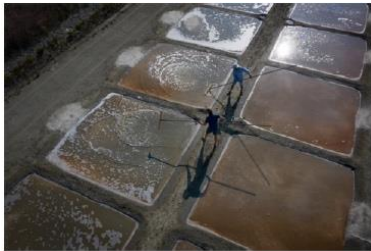
Figure F.11. Ile de Ré: coarse salt is moved with water pushed with the simoussi (Merlin 2020)
