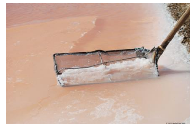
Figure F.17 Flor de Sal skimmed off in a crystalliser, Eastern Algarve, Portugal
