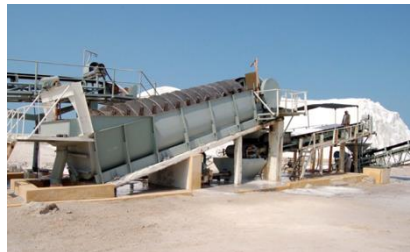
Figure F.29. Sea salt washing facility, from Sedivy Vladimir, processing of salt for human and industrial consumption, 2009
