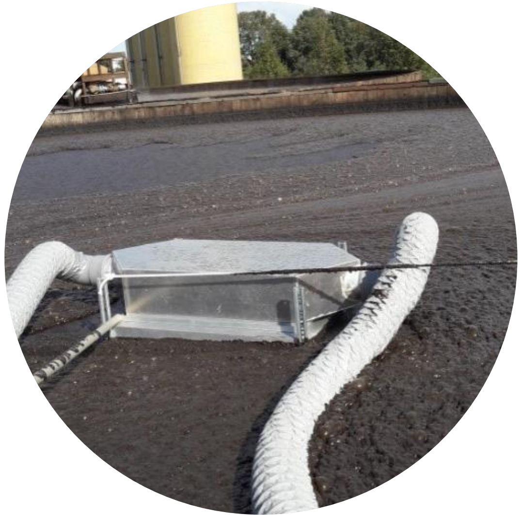
Measurement on a nitrification/denitrification unit with floating Lindvall box
